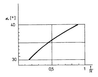
$\frac{\text{Fig.3}}{\text{ness t }}$  Dependence of crack propagation direction on sphere thickness t (R = radius of the sphere)
