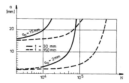
Fig.4 Remaining fatigue life of the spherical joint for two limiting thickesses t (a = initial crack length, N = number of cycles)
