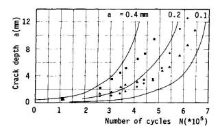
Figure 9 Crack growth data for part-through cracks, position (2), cf. Fig.1
