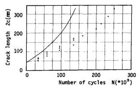
Figure 10 Crack growth data for through-thickness cracks, position (1), cf. Fig.1
