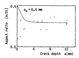
Figure 7 Crack shape data for part-through cracks at external stiffener welds (Position (2), cf. Fig.1)
