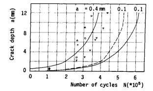
Figure 8 Crack growth data for part-through cracks, position (1), model no. 2
