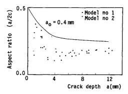
Figure 6 Crack shape data for part-through cracks at brace/column weld (Position (1), cf. Fig.1)
