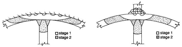
Figure 3 Stages of crack growth at brace/column welds
