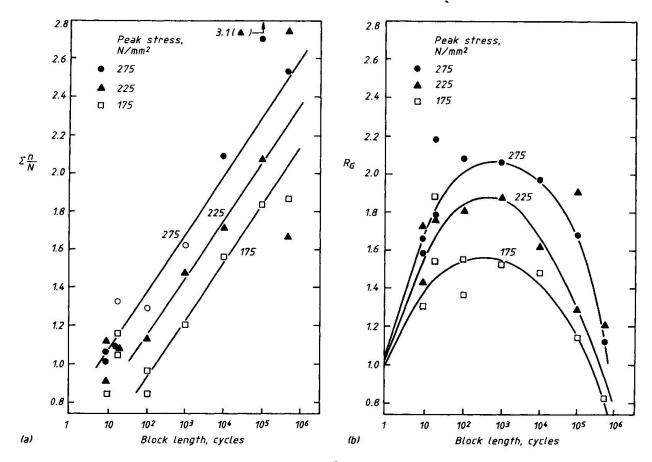
$\underline{\text{Fig.6}}$  Influence of block length on (a)  $\Sigma_{\overline{N}}^{\underline{n}}$  and (b)  $R_{\overline{G}}$  for Rayleigh spectra
