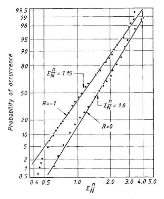
Fig. 9 Effect of R on values of  $\Sigma_{N}^{n}$  for block programme tests
