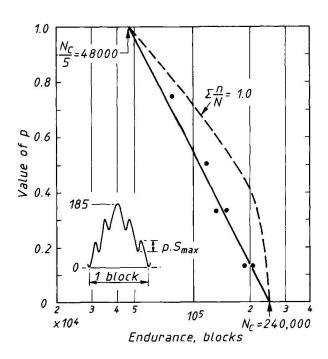
Fig.3 Typical results obtained using simple stress sequences
