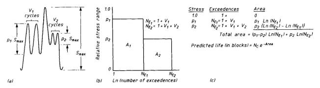
Fig. 4 Example of life calculation using the area rule
