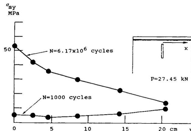
Fig.11 Distribution of web surface stress  $\sigma_{sy}$  along the flange-to-web fillet weld (Specimen B-1)
