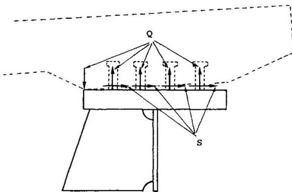
**Fig.13** Forces acting on F.E.M. model
