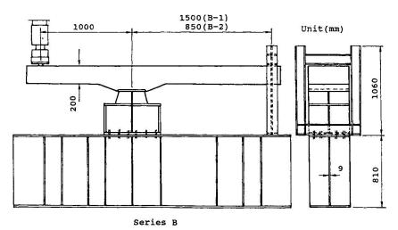
Fig.9 Fatigue test specimens
