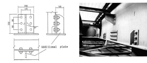
Fig. 10 Retrofitting by additional plate
