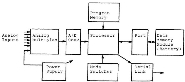
Fig. 2 Block diagram of the device
