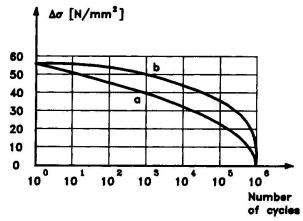
Fig.1 Stress collective: a) narrow band and b) wide band structural response
