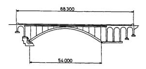
Fig. 5 Bridge E: Deck type arch bridge
