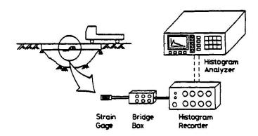
Fig. 6 Measurement of stress histogram
