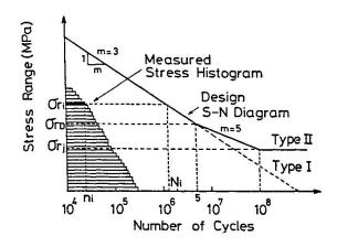
Fig. 8 ECCS design S-N diagram
