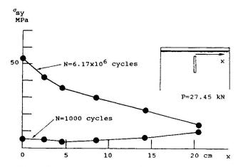
Fig.11 Distribution of web surface stress  $\sigma_{\rm SY}$  along the flange-to-web fillet weld(Specimen B-1)
