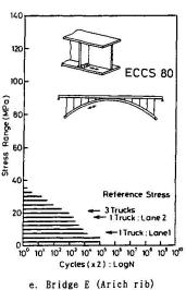
Fig. 7 Example of stress range histogram records
