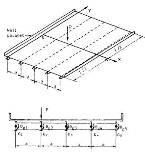
Fig.4 Concrete slab under concentrated load P
