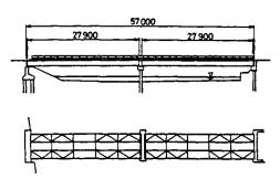
Fig. 2 Bridge B: Composite plate girder bridge
