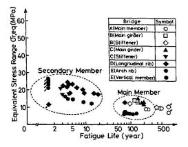
Fig. 10 Equivalent stress range and fatigue life for Bridges C, D and E
