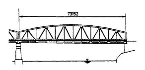
Fig. 1 Bridge A: Riveted truss bridge
