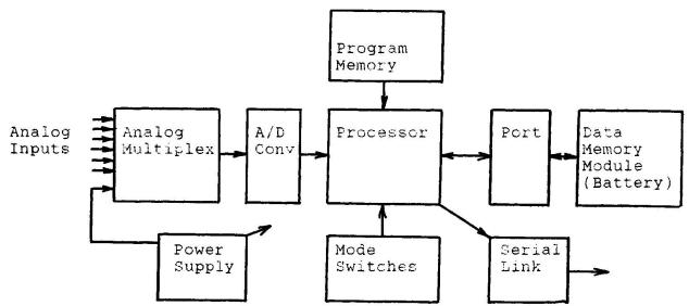
Fig. 2 Block diagram of the device
