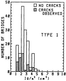
Fig.7 Relationship between I<sub>O</sub>/a<sup>2</sup> and the number of bridges in which Type 1 cracks were observed
