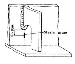
Fig.6 Position of strain gauge
