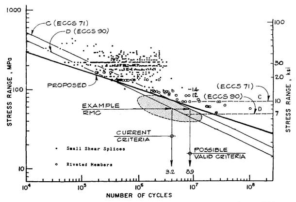
Comparison of fatigue resistance of full-size members with small shear splices. (3, F16.32)
