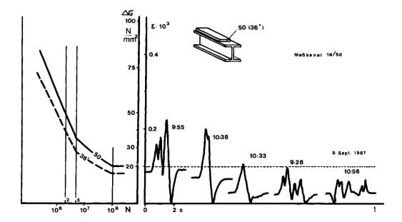
Figure 5. Measured strains/stresses during about 3 hours of observation at one measuring point.
