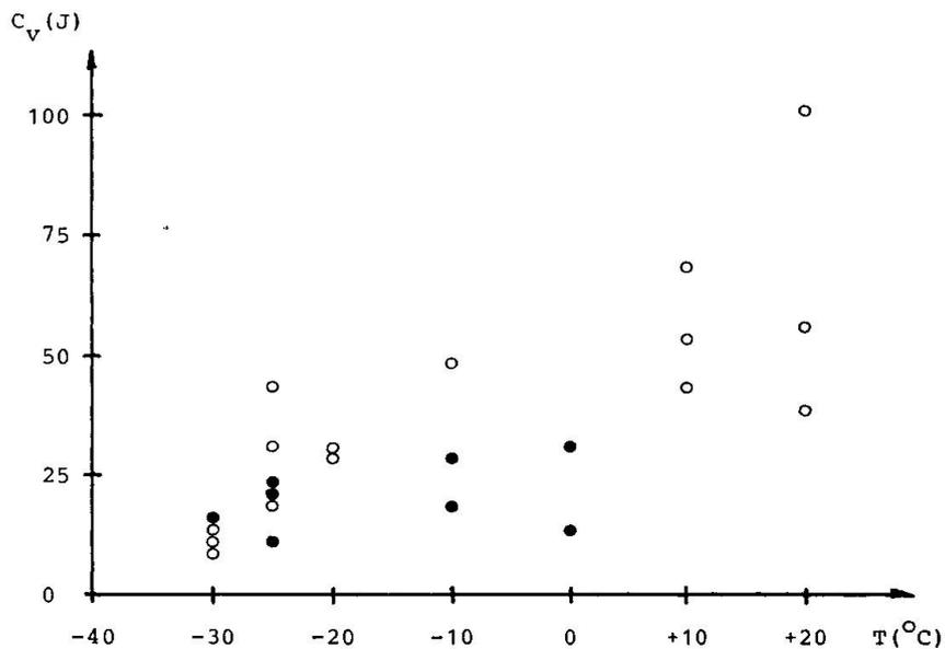
Fig 1. Charpy-V notch toughness for two specimen series of a given material. o Ser no 1. ● Ser no 2.
