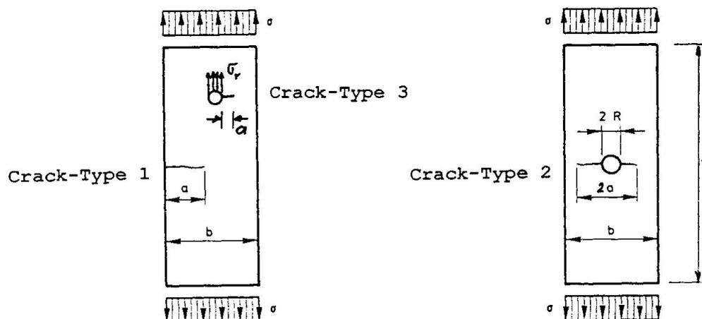
Fig. 9: Definition of crack-types 1, 2 and 3 considered in Tab.3.
