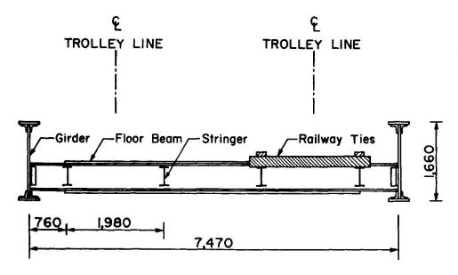
Fig. 1 Cross Section of Trolley Bridge
