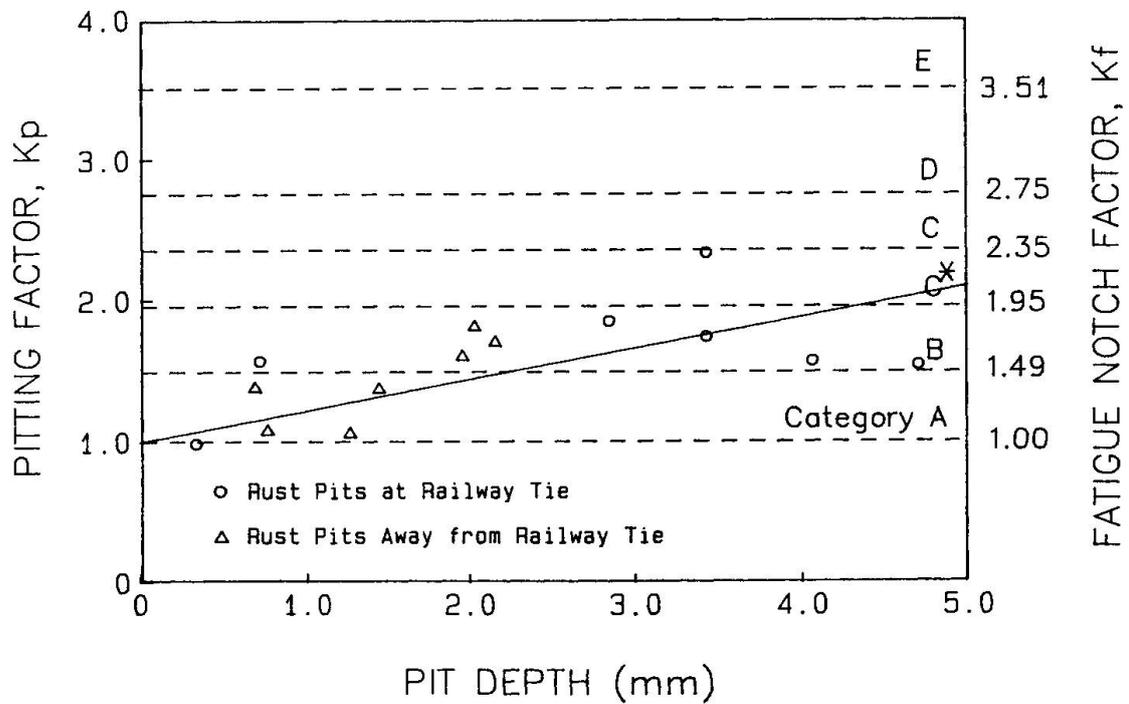
Fig. 7 Pitting Factor for Carbon Steel Beams
