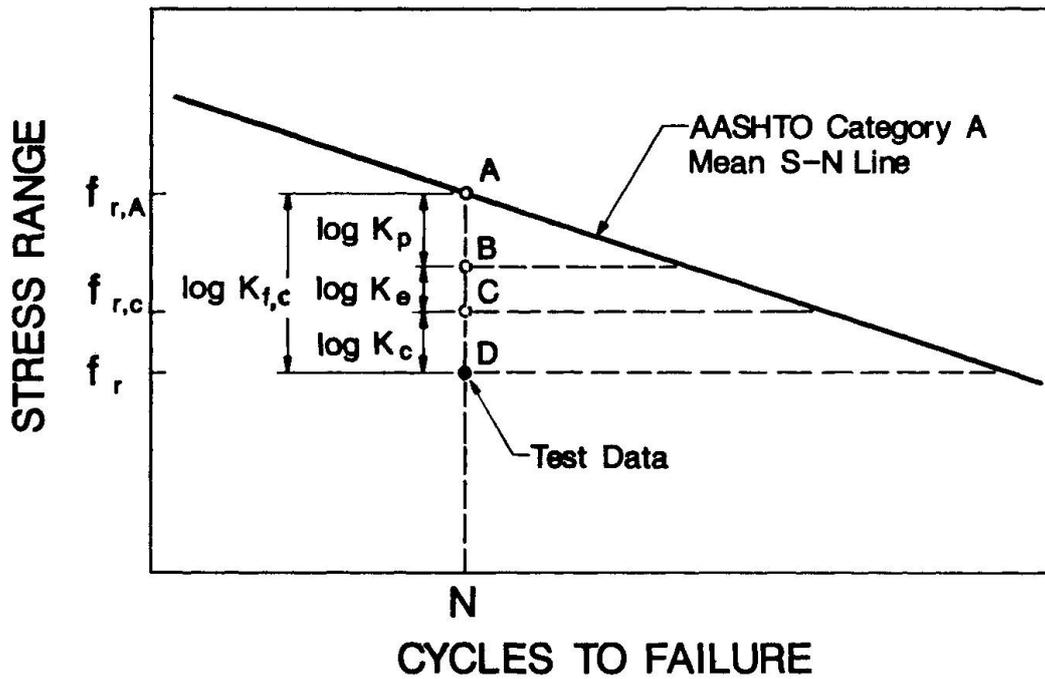
Fig. 4 Illustration of Fatigue Strength Reduction Factors
