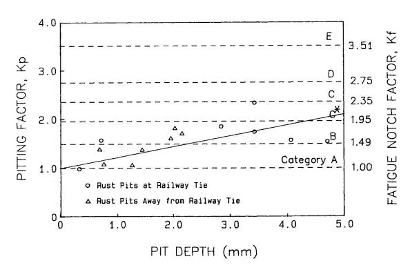
Fig. 7 Pitting Factor for Carbon Steel Beams
