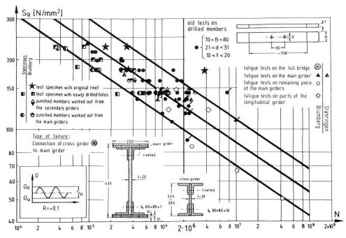
$\frac{\text{Fig. 8}}{\text{est}}$  Results of tests on components of the Blumberg bridge compared to earlier test results of punched specimens
