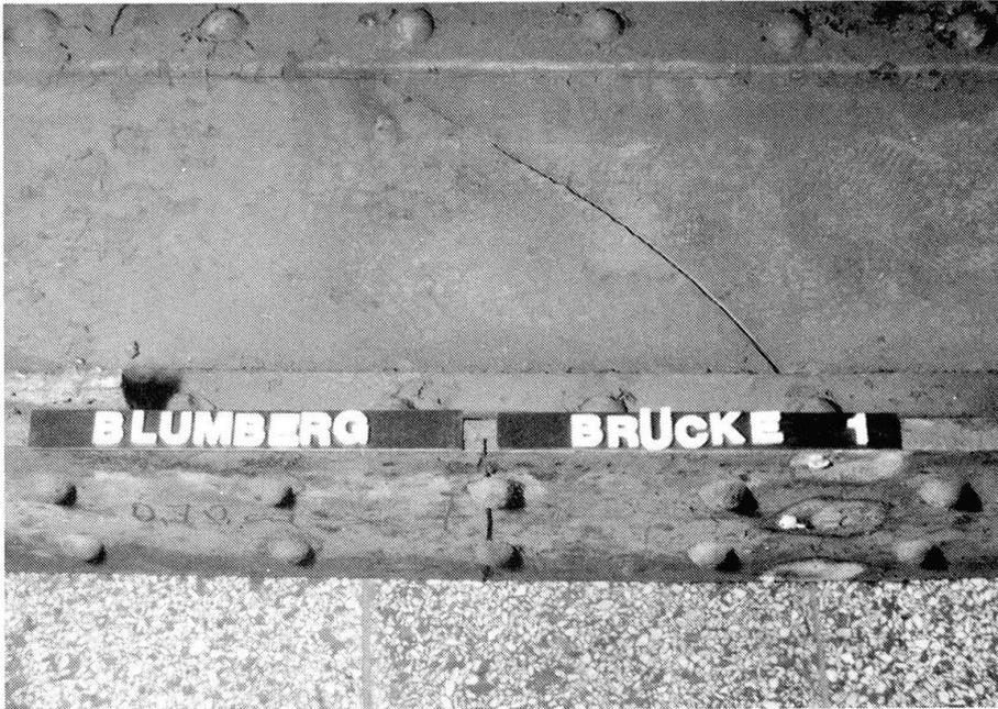
Fig. 7 Points of fracture of main girder I
