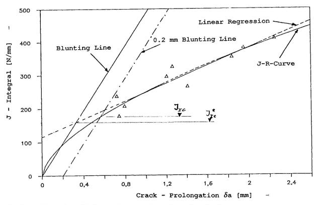
Fig. 5: Example of J-Integral vs. crack-prolongation  $\delta a$  (J-resistance-curve) calculated from load-displacement-curve (Fig. 4) and definition of  $J_{1c}$  For comparision  $J_{1c}$  according to ASTM E813-81 (issue 1981 of [7]), denoted by  $J_{1c}^*$ , is also shown.
