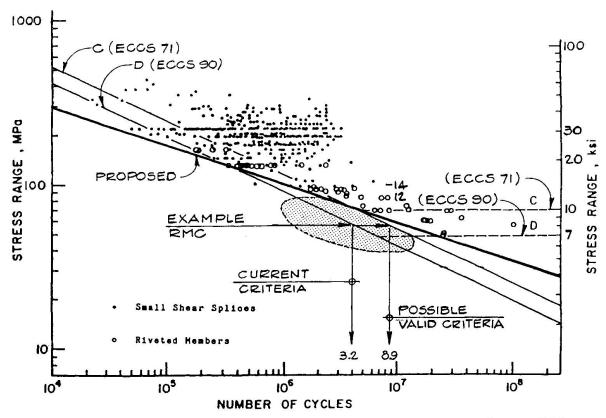
Comparison of fatigue resistance of full-size members with small shear splices. (3, F16.32)
