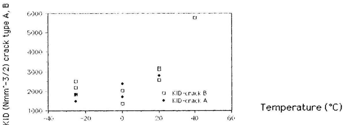
Fig. 7: Dynamic fracture toughness vs. temperature
