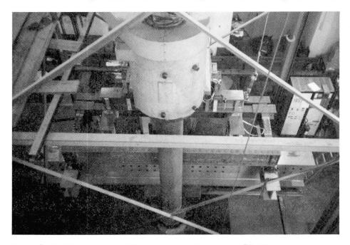
Fig. 3 Bridge of the "Museumsbahn" in the 50 MN power press
