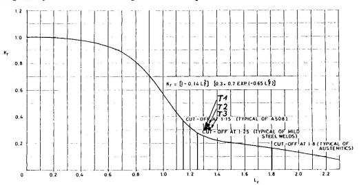
Fig. 8: Failure assessment diagram according to [12]. The points T1, T2 and T3 correspond to fracture tests on precracked component—like specimens
