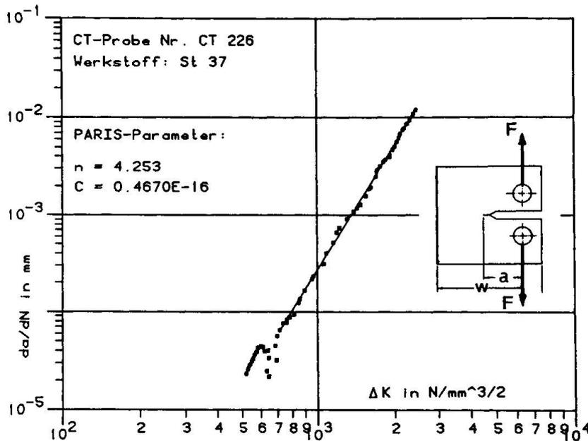
Figure 3. Result of one of the crack growth tests (ASTM E 647-83) with regression line regarding the Paris equation (1)
