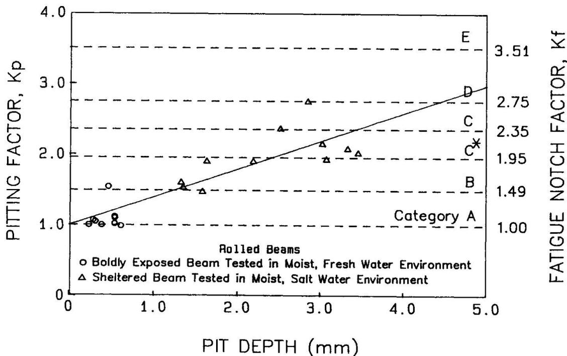
Fig. 8 Pitting Factor for A588 Weathering Steel Beam
