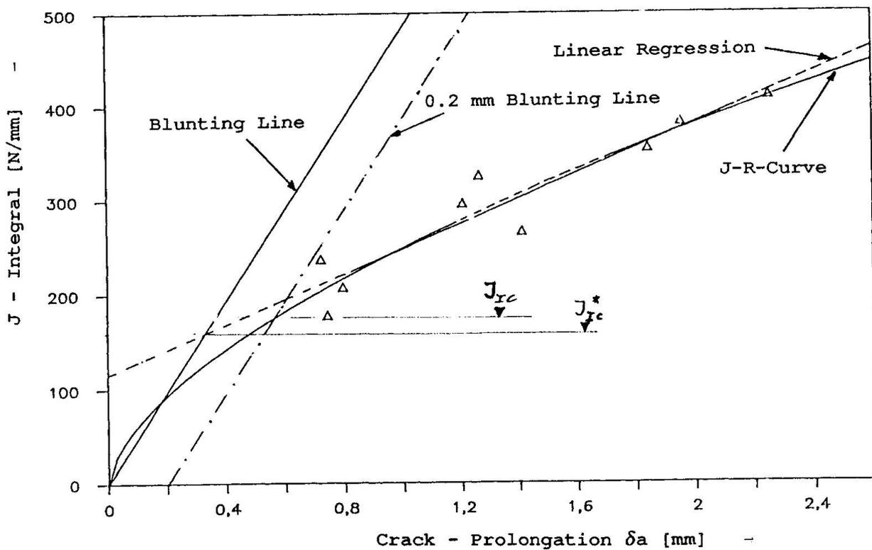
Fig. 5: Example of J-Integral vs. crack-prolongation  $\delta a$  (J-resistance-curve) calculated from load-displacement-curve (Fig. 4) and definition of  $J_{1c}$ . For comparison  $J_{1c}$  according to ASTM E813-81 (issue 1981 of [7]), denoted by  $J_{1c}^*$ , is also shown.
