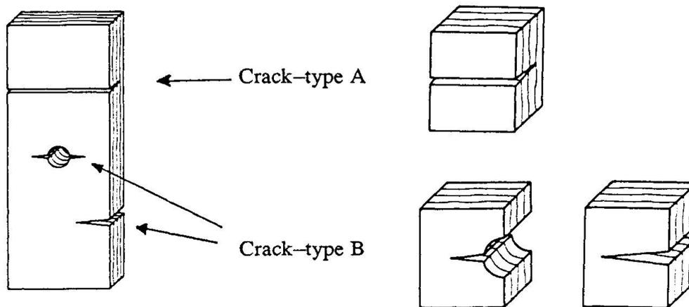
Fig. 2: Definition of crack-type A resp. B.
