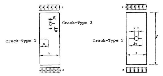
Fig. 9: Definition of crack-types 1, 2 and 3 considered in Tab.3.
