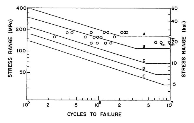
Fig. 2 Fatigue Test Data for Carbon Steel Beams
