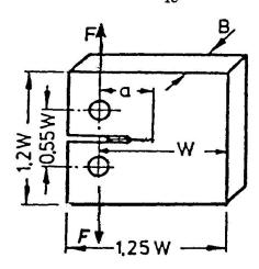
Fig. 3: Geometry of compact tension (CT-) specimen used. For dimensions see Tab. 2.
