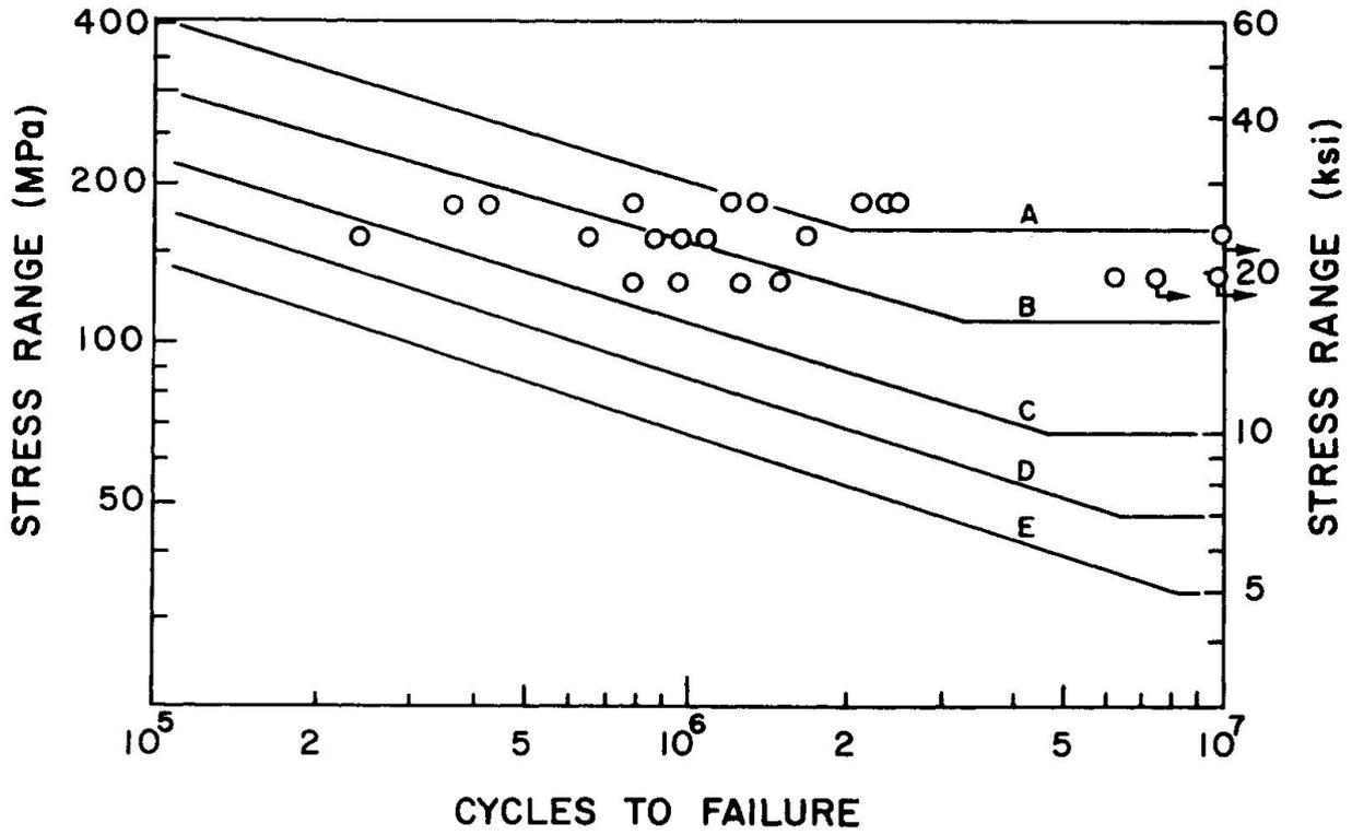
Fig. 2 Fatigue Test Data for Carbon Steel Beams
