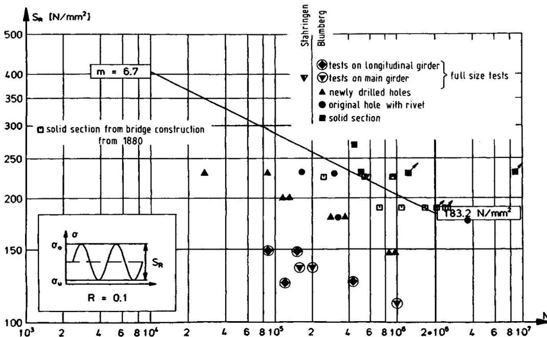
Fig. 15 Test results and data from [5], bridges dating from 1880, plain material prestressed by 290 N/mm<sup>2</sup> and 10<sup>5</sup> stress cycles
