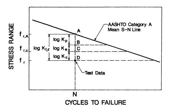
Fig. 4 Illustration of Fatigue Strength Reduction Factors
