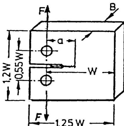
Fig. 3: Geometry of compact tension (CT-) specimen used. For dimensions see Tab. 2.
