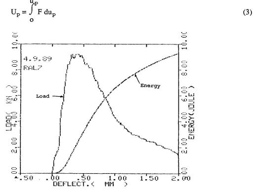
Fig. 6: Example of a load vs. deflection curve and transmitted energy vs. deflection curve of a 3-point-bend impact test with precracked Charpy-specimen. This curve is calculated from the load vs. time curve.
