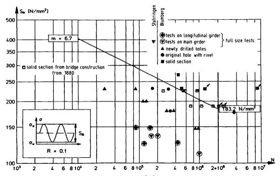
Fig. 15 Test results and data from |5|, bridges dating from 1880, plain material prestressed by 290 N/mm<sup>2</sup> and 10<sup>5</sup> stress cycles
