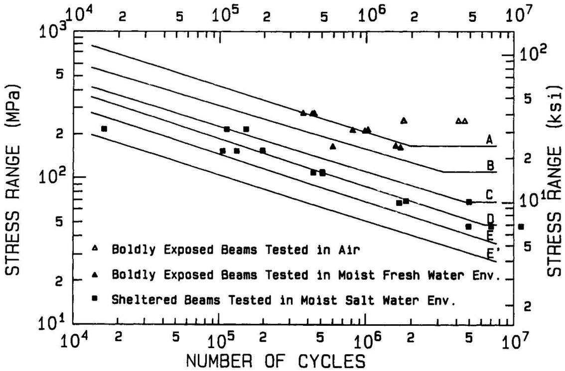
Fig. 3 Fatigue Test Data for Weathering Steel Beams
