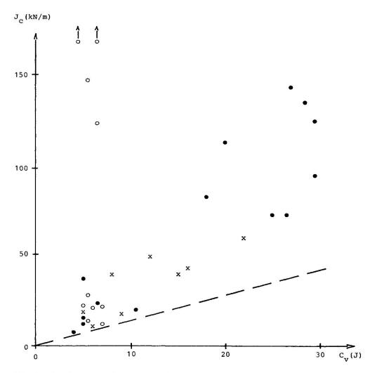
Fig 2. Fracture toughness J and Charpy-V notch toughness C o This investigation, x Ref (4),  $\bullet$  Ref (5).
