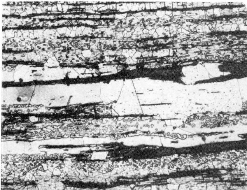
Fig. 1: Microstructure of wrought iron (magn. 50x)
