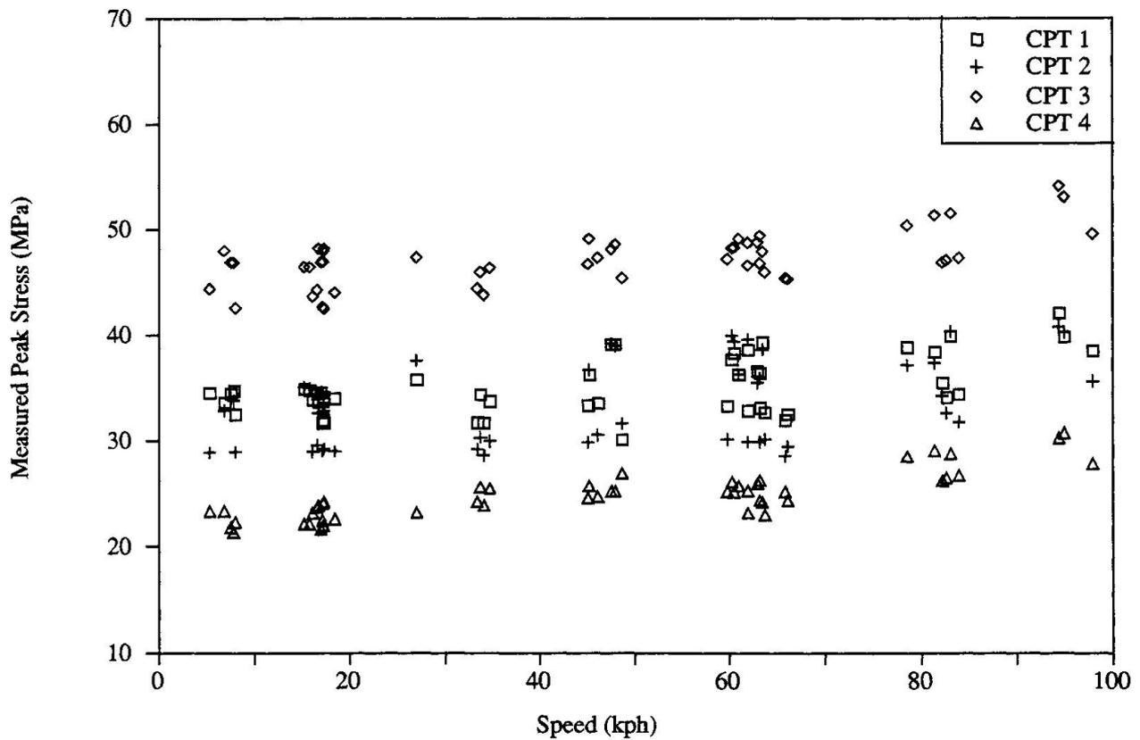
Figure 3 - Stresses at coverplate terminations, 9.9 m span at Mangalore
