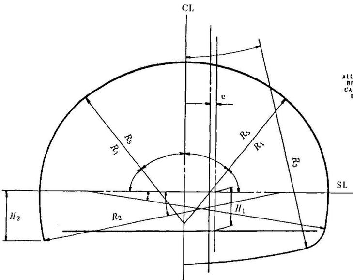
Fig. 4: Definition of dimensions of a tunnel
