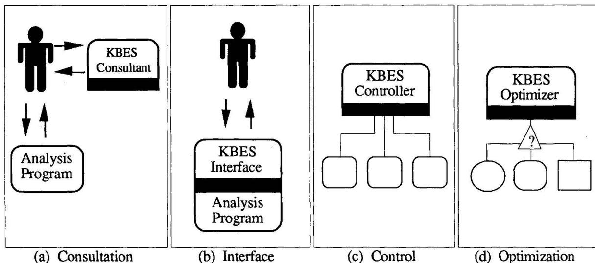
*Fig. 2* KBES Applications to Finite Element Analysis.
