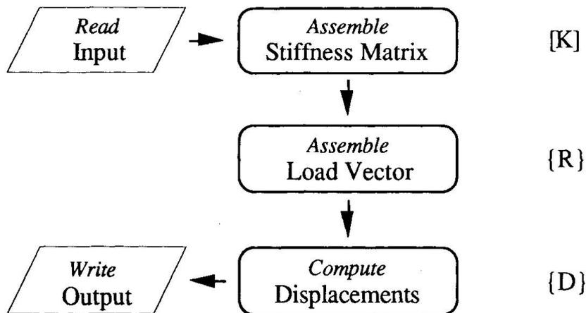
*Fig. 1* Displacement Computation Algorithm.
