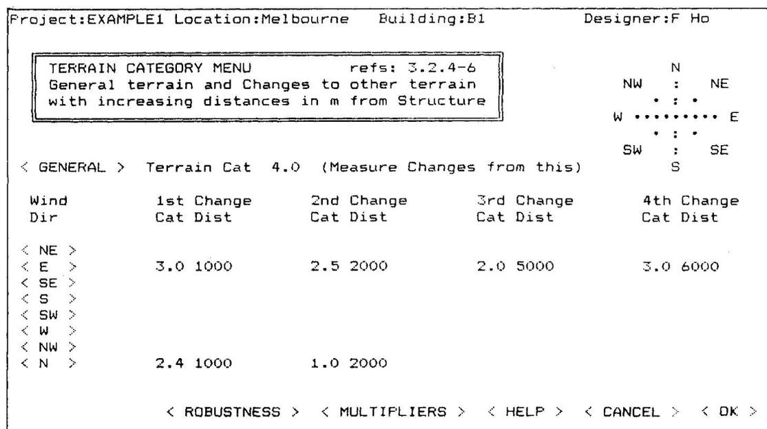
Fig. 2. Input screen for input and checking Terrain Category and changes.
