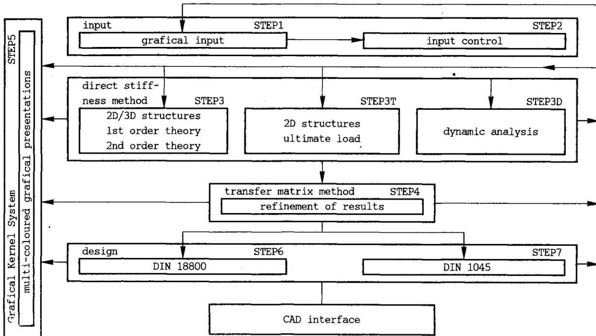
Fig 1: Modular structure of the program system SSt-micro [6]
