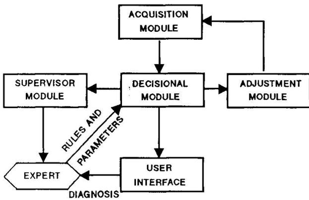
The acquisition module allows the periodical and automatic collecting of measurements obtained by the different monitoring subsystems (hydrological, geotechnical). The data which are not acquired automatically are handled manually by means of controlled video masks. The programs check the validity of measurements in order to transmit only reasonable measurements to the DECISIONAL MODULE.
