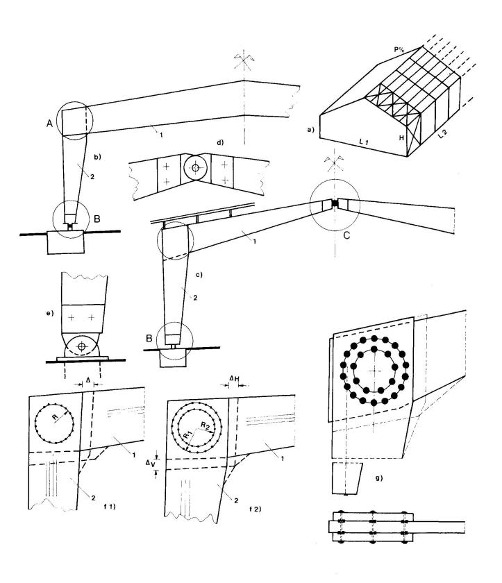
Fig. 3. a) The outlines of the building, b), c) the two and three hinged glulam frame, d) the top joint of the three hinged frame, e) detail of the support hinge, f), g) details of the generated circular bolted corner joint (one or two rings).
