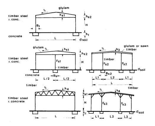
Fig. 2. An early 2D optimization approach to different structural systems.
