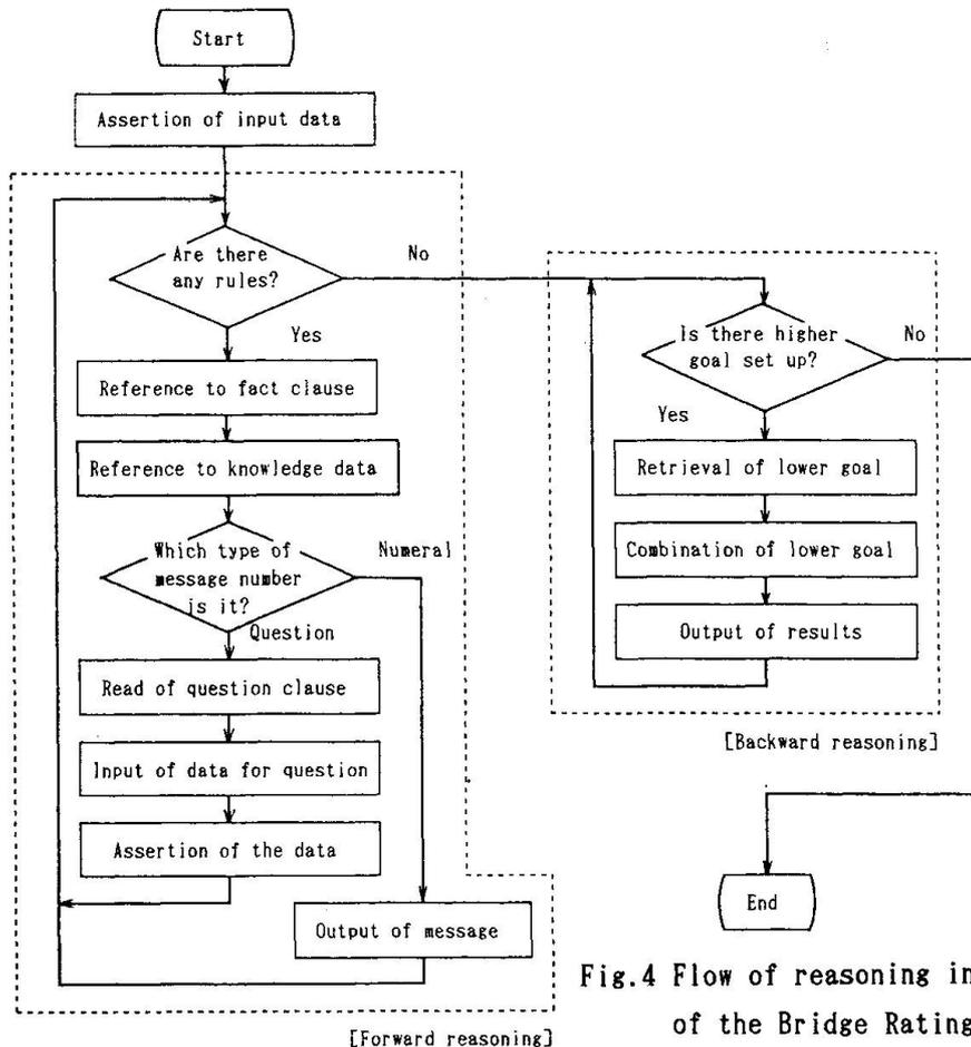
Fig.4 Flow of reasoning in inference engine of the Bridge Rating Expert System
