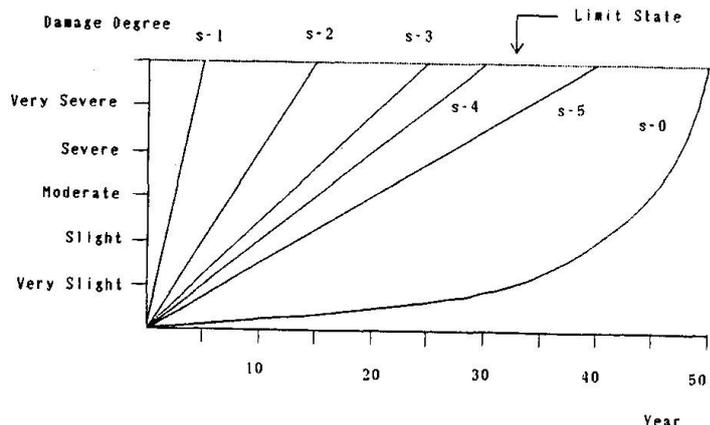
Fig. 3 Relation between construction year and damage state
