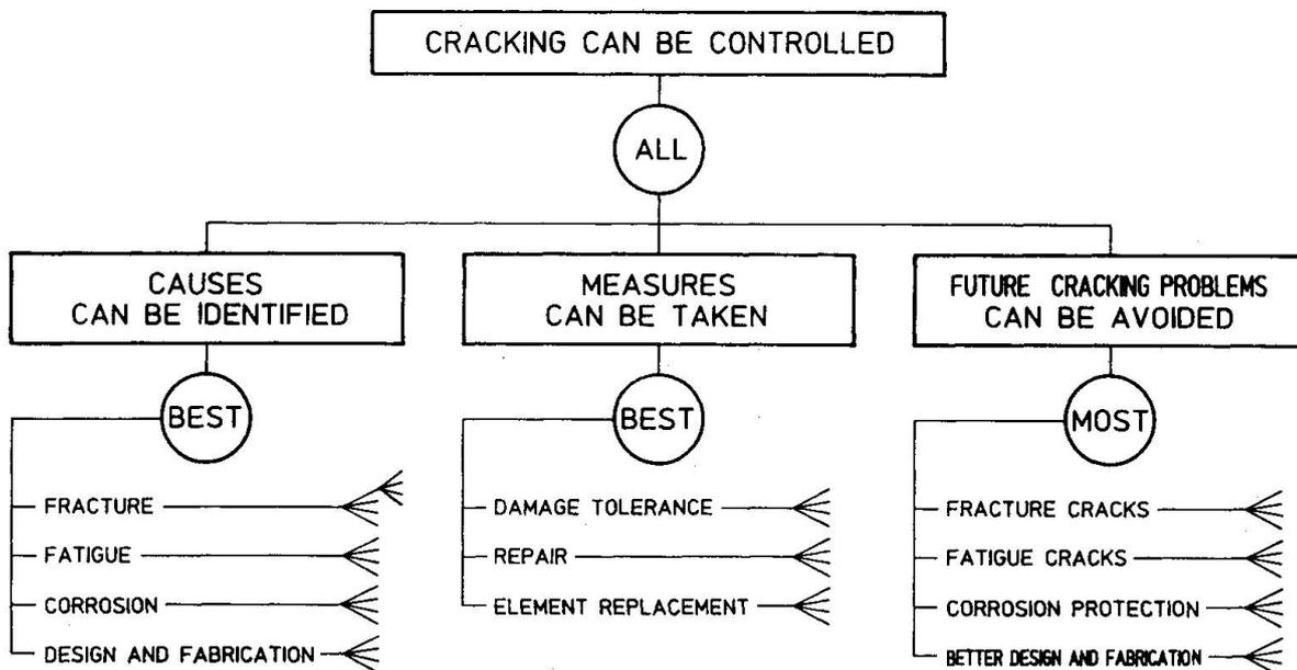
FIGURE 2 *Partial inference net of CRACK CONTROL*
