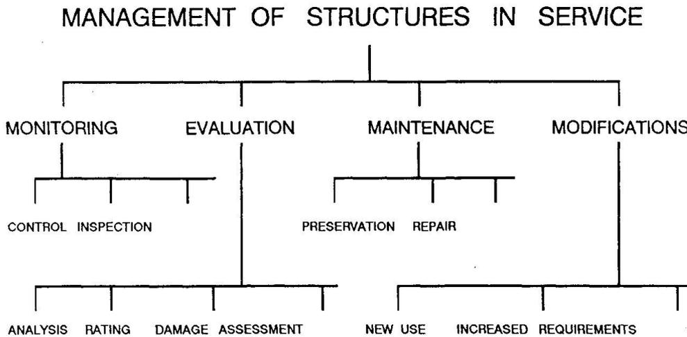
FIGURE 1 *Activities associated with the management of structures in service*
