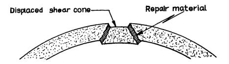
Figure 1. Sectional view of a dome repair
