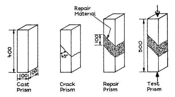
Figure 3 Cementicious grout bonded slant shear test method
