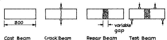
Figure 5 Recommended flexural test for resin or cementicious bonded beams
