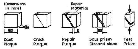
Figure 2 Resin bonded slant shear test method
