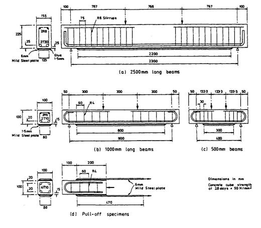
Fig. 1 Details of Test Specimens
