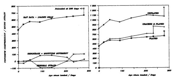
Fig. 3 Strain Data for Plated Beam
