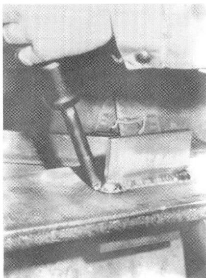
FIGURE 3 : Improvement methods, particularly hammer peening, may increase fatigue strength.
