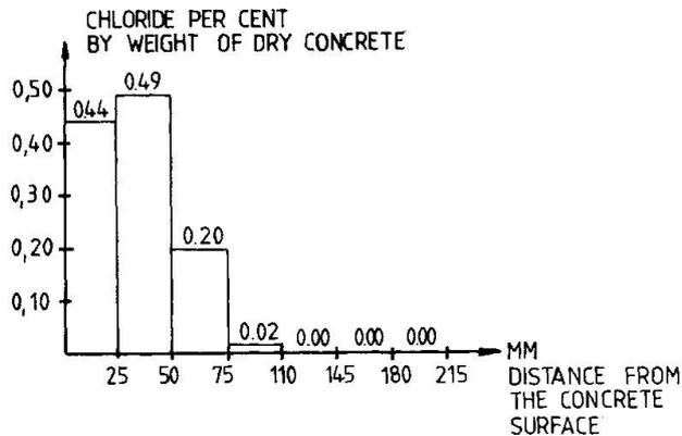
Fig. 2 Typical Chloride Profile at Ground Level
