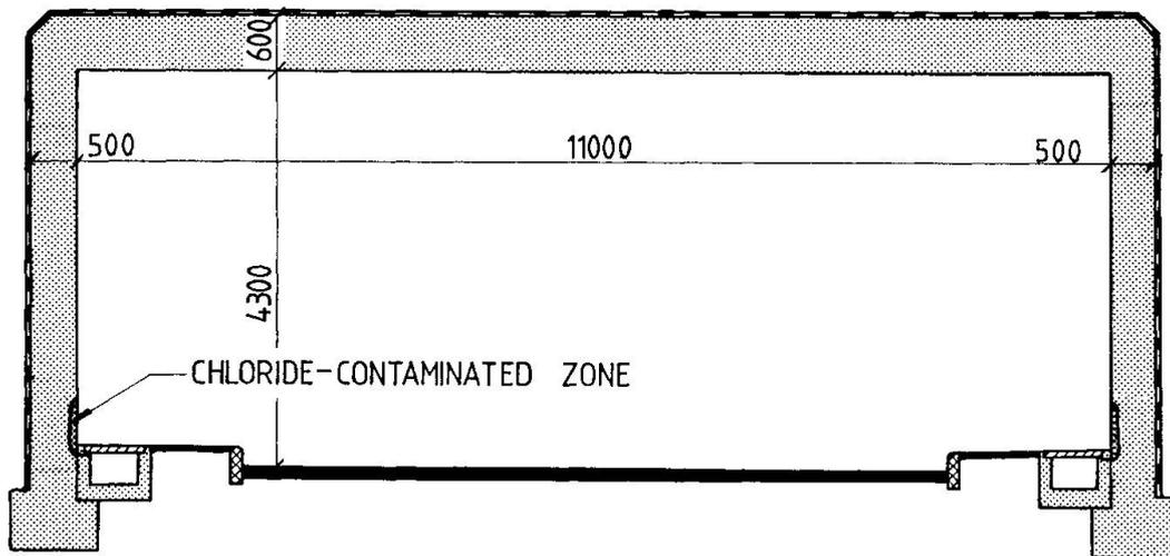
Fig. 1 Cross Section of Tunnel
