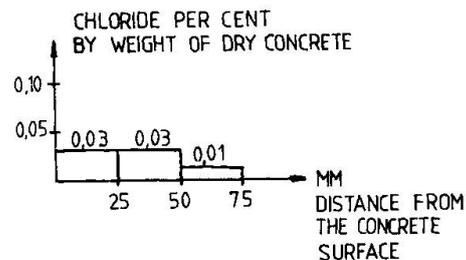
Fig. 3 Typical Chloride Profile approx. 0.7 m above Ground Level
