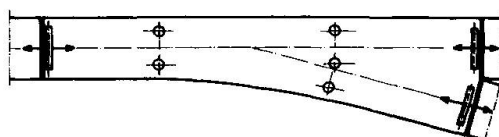
Fig. 7 - Irregular disposition of expansion bearings
