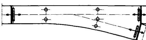
Fig. 7 - Irregular disposition of expansion bearings
