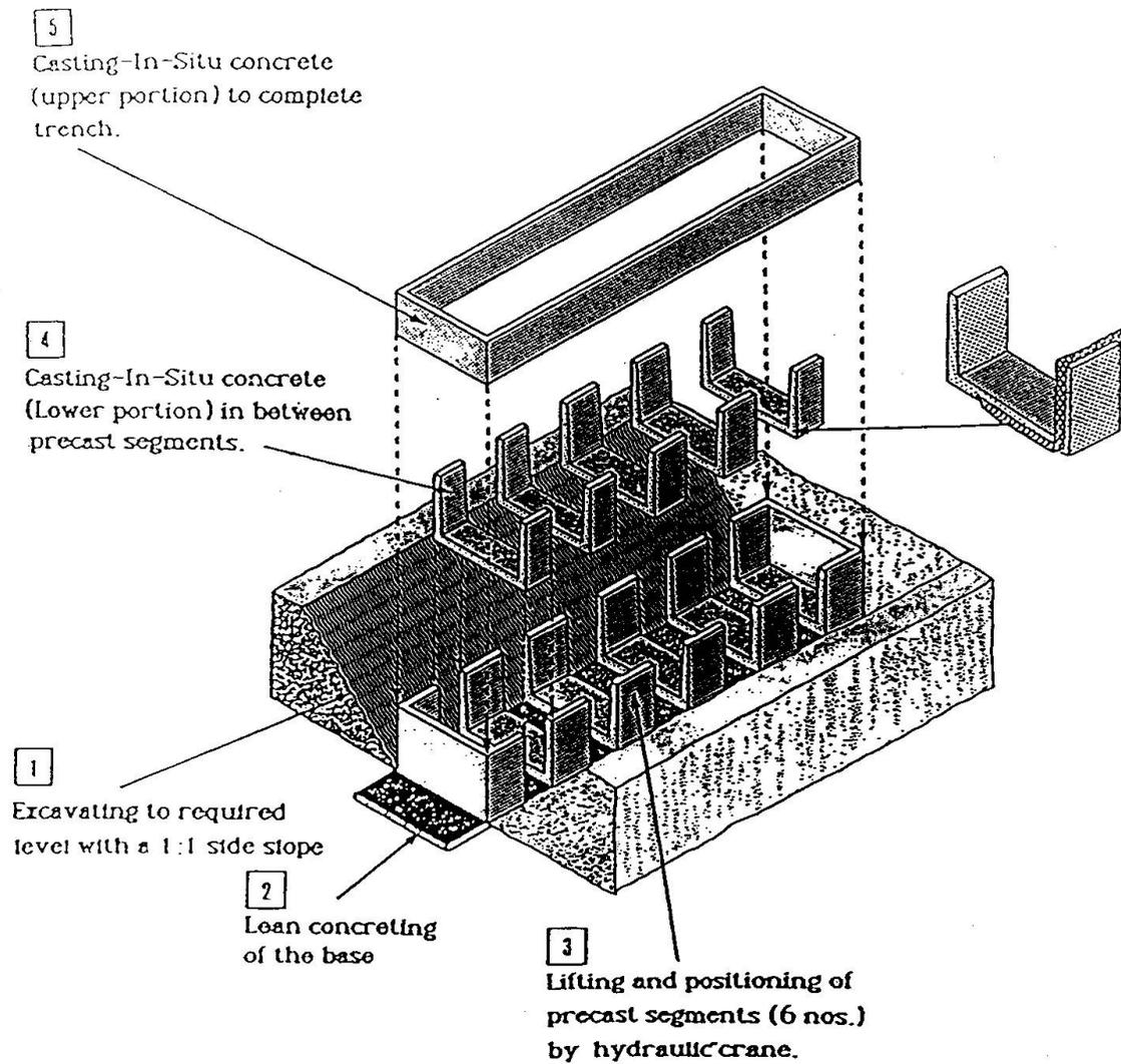
Fig.1 Sequence of construction
