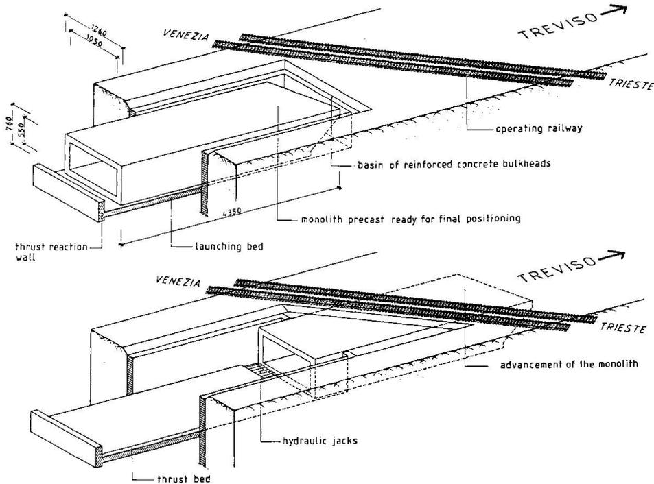
Fig. 5 - Scheme of the positioning operations
