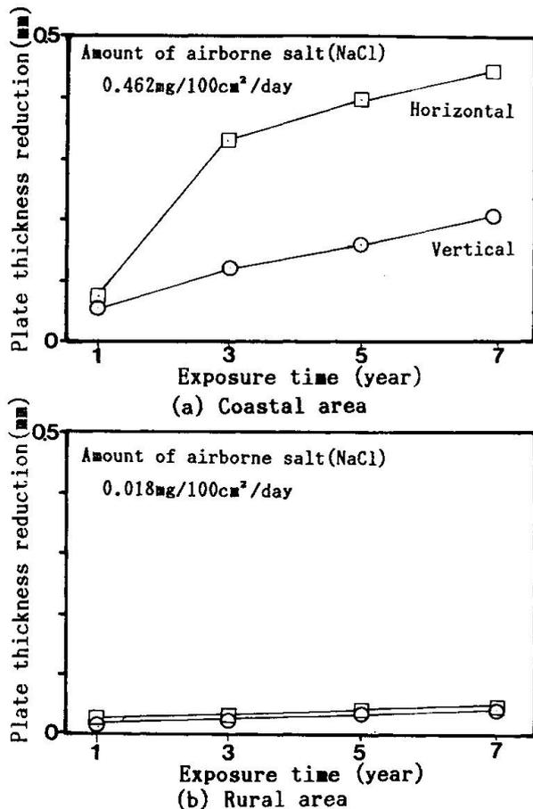
Fig.2 Annual change in plate thickness reduction
