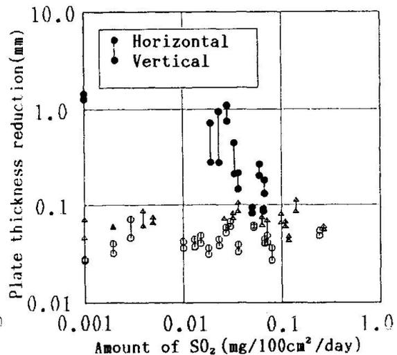
Fig.4(b) The relation between the plate thickness reduction after 7 years exposure and the amount of SO<sub>2</sub>
