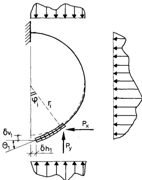
The flexural stiffness of the pipe-wall varies along the circumference, which effects the internal distribution of the loads.
