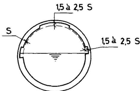
Fig. 1 Schematization of the deterioration of the pipe-wall
