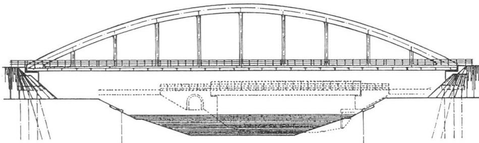
Fig 1 Tied arch with vertical suspension hangers
