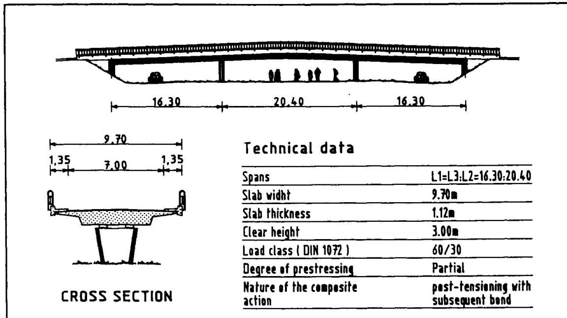
Fig. 5 Triple span roadbridge
