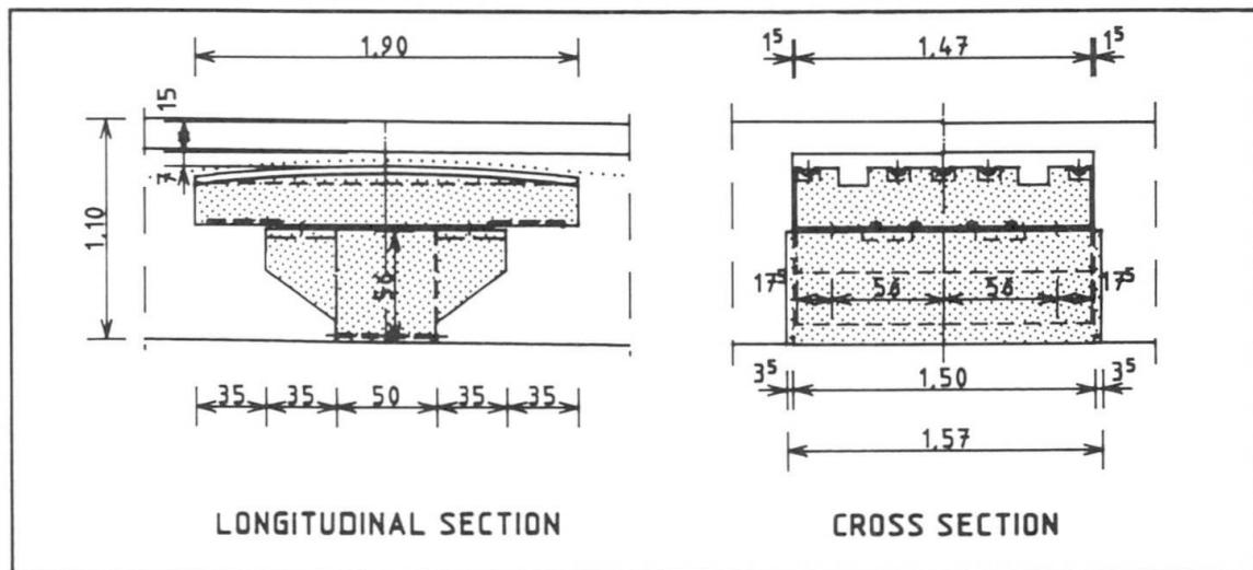
Fig. 3 Diversion support for the prestressing tendons
