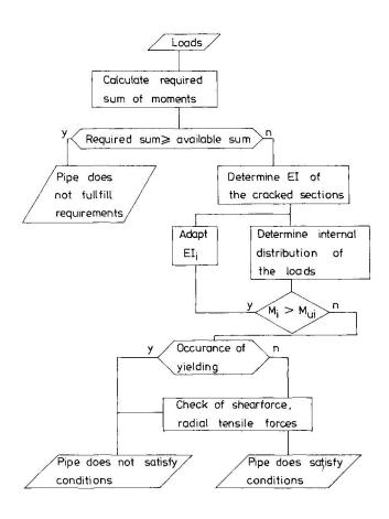
Fig. 6 Flow diagram design model
