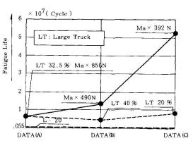
Fig. 8 Influence to Fatigue Life due to Max Truck Weight and Occurrence Ratio of Large Truck
