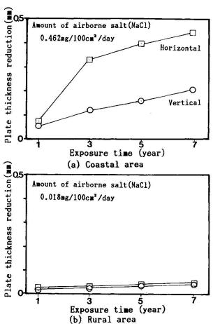
Fig. 2 Annual change in plate thickness reduction
