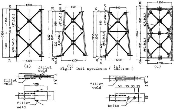
Fig.2 Welded connection
