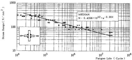
Fig. 3 Fatigue Properties for Load -Carrying Cruciform Welded Joints
