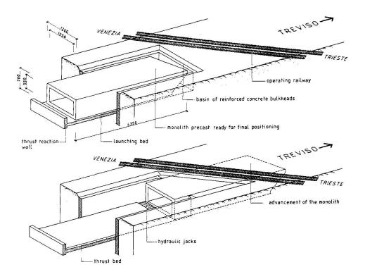
Fig. 5 - Scheme of the positioning operations
