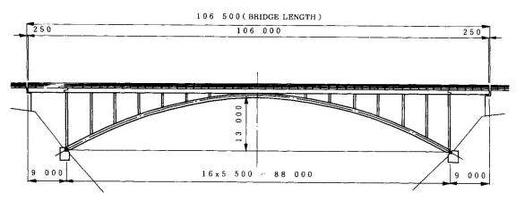
Fig. 1 General View of Deck Arch Bridge
