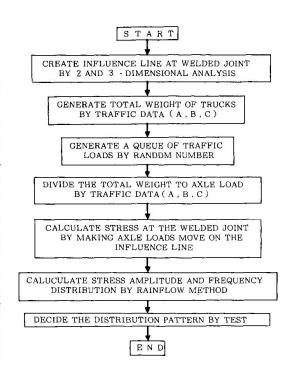
Fig. 4 Flow Chart of Fatigue Analysis
