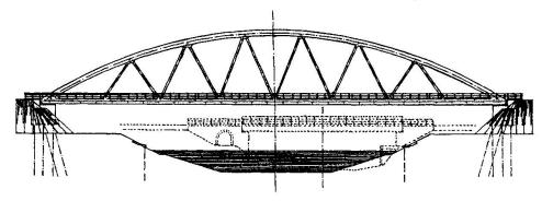
Fig 3 Further improvement of triangulated hangers tied arch
