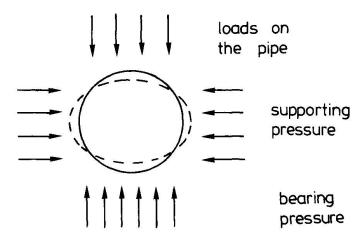
Fig. 2 Behaviour of a relatively flexible pipe
