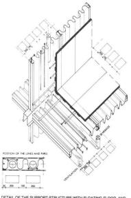
DETAIL OF THE SUPPORT-STRUCTURE WITH FLOATING-FLOOR, AND PREPOSITIONED WALL-PANELS
