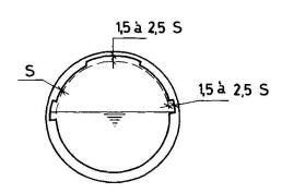
resulting in a decrease of the thickness of the pipe wall. This deterioration takes place - as opposed to other mechanism - above the water-level and is not uniformly distributed along the inside of the pipe. As approximate guide values for the deterioration at the top and the water-level are given 1,5 times respectively 2,5 times the mean value [3]. See figure 1.
