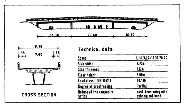
Fig. 5 Triple span roadbridge
