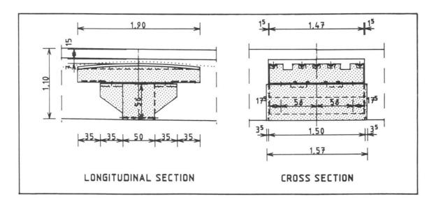
Fig. 3 Diversion support for the prestressing tendons
