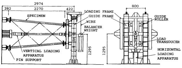
Fig.4 Loading apparatus (unit;mm) P(kN) P(kN) 150 100 100 50 50 Ø -5D -50 -100 -100 -150 10 5 D(cm) D(cm) Type-AB P-D relation. Fig.5 Type-AW P-D relation Fig.6
