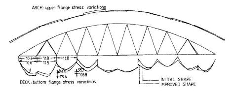
Fig 4 Reducing of stress fluctuations by optimizing
