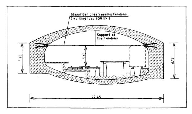
Fig. 4 Cross section of the subway station in Paris
