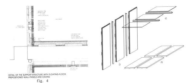
With the so obtained support system, consisting of 4 subsystems each with very few different elements, it is possible to build up a wide scale of different supports for all types of dwellings.
