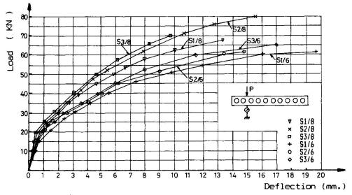
$\underline{\text{Fig. 4}}$  Load deflection curves of the six tested slabs for a point under the load ( Eccentric loading ).
