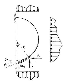
Fig. 4 Arc of circle restrained
