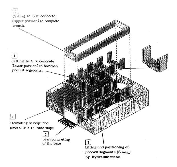
Fig.1 Sequence of construction
