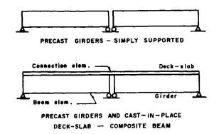
Fig. 3.1 - Deck-Continuous Beam
