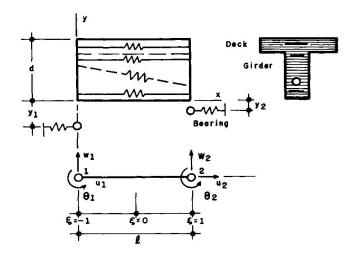
Fig. 2.1 - Beam element
