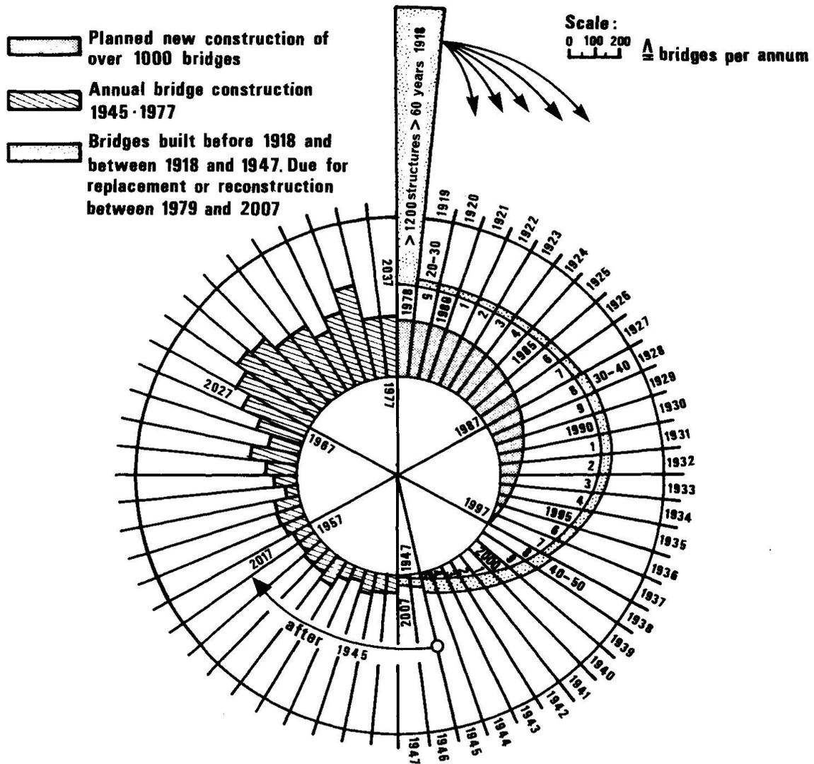
Fig. 2 : Bridge generation cycle of Rhine Palatinate Land
