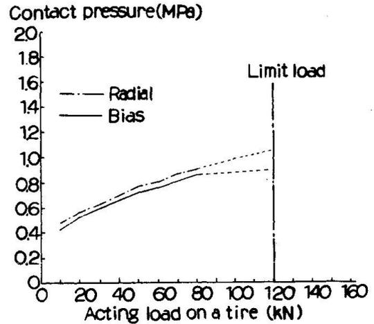
Fig.4 Acting load and contact pressure relation
