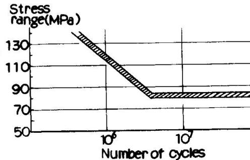
Fig.7 S-N Curve of aluminium alloy (A-S7G06) [4]
