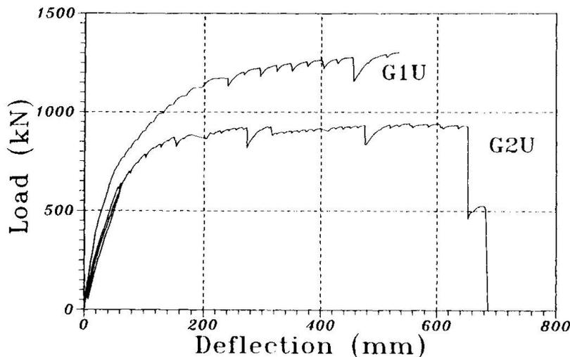
Figure 4 - Load-deflection curves for ultimate tests.
