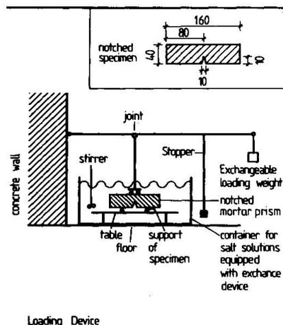
Fig.1: Loading Device for Stress Corrosion Tests
