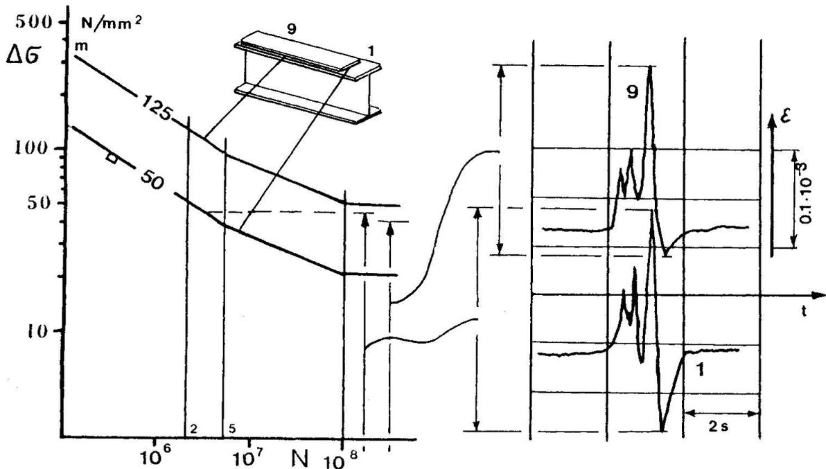
The crack growth tests offered the possibility to assess the amount of growing of a crack of a certain length which was not detected during an inspection within the time interval up to the next inspection (3 years). From the measurements, it turned out that the cracks (fig. 4) were caused by residual forces.
