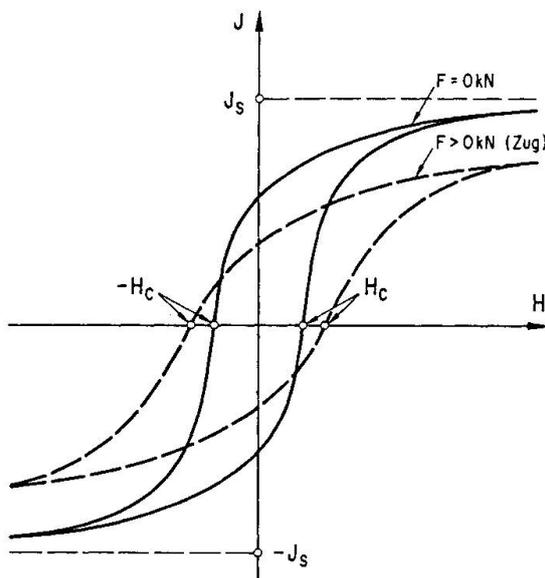
Fig.1 Magnetoelastic effect on prestressing steel
