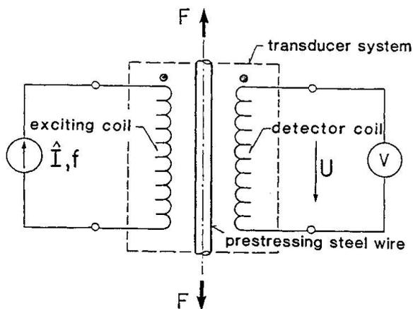
Fig.2 Magnetoelastic F-measurement
