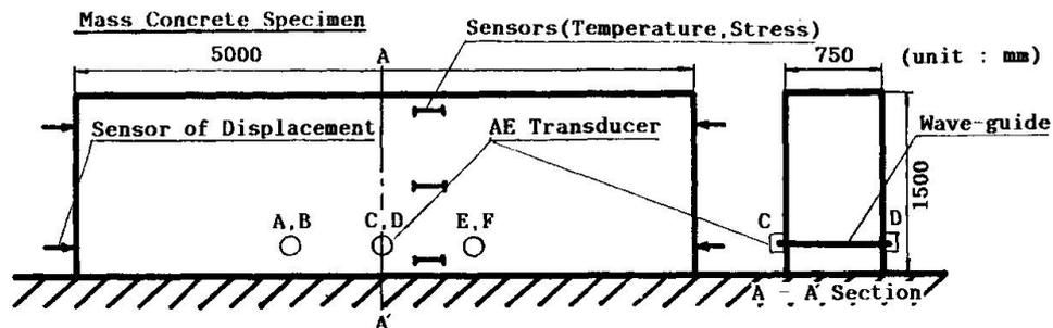
Fig. 1 Mass Concrete Specimen and Locations of Sensors
