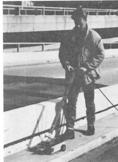
Fig. 2 Guiding the radar antenna for the detection of transverse prestressed reinforcement
