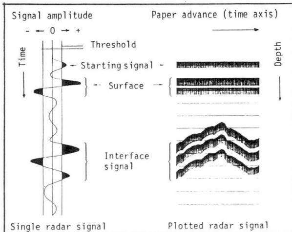
Fig. 1 Graphic recording of a radar signal.
