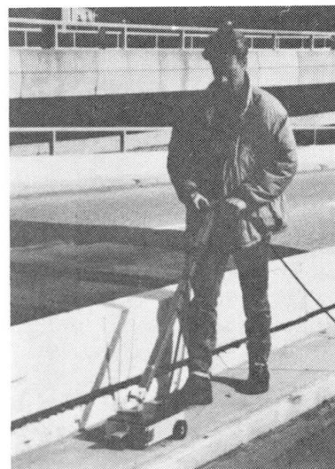
Fig.2 Guiding the radar antenna for the detection of transverse prestressed reinforcement
