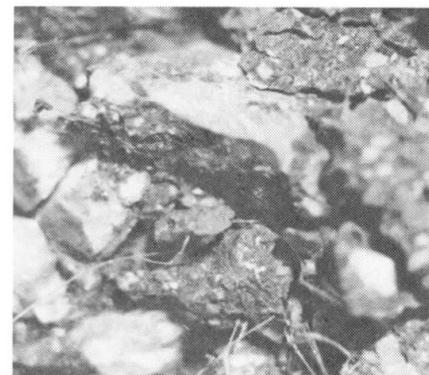
Fig.8 Distribution of fibers in hardened concrete
