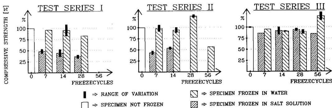
Fig. 2: Results of static compressive strength tests
