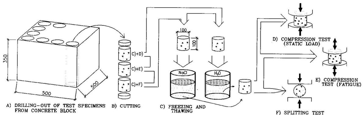
Fig. 1: Test procedure
