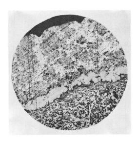
Fig. 2 Aluminum coating microstructure
