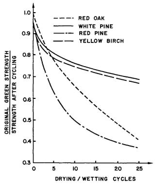
Fig. 2 Influence of Drying-Wetting Cycles on Shear Strength
