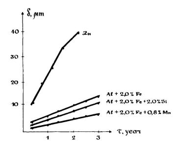
Fig. 1 Dependence of the values of corrosion failure (6) of aluminum and zinc coatings of steel upon the test period (7) in conditions of an integrated chemical plant
