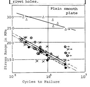
Fig.3 Results of Fatigue test of Cumulative Damage
