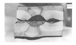
Fatigue Crack of Lower Flange of Beam Specimen (B)
