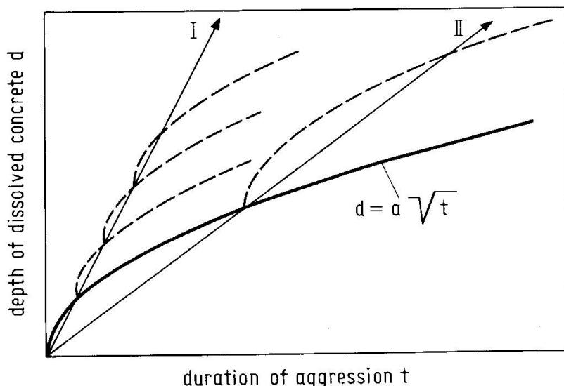
Fig. 1 Acceleration of a solvent attack when removing the protective layer periodically
