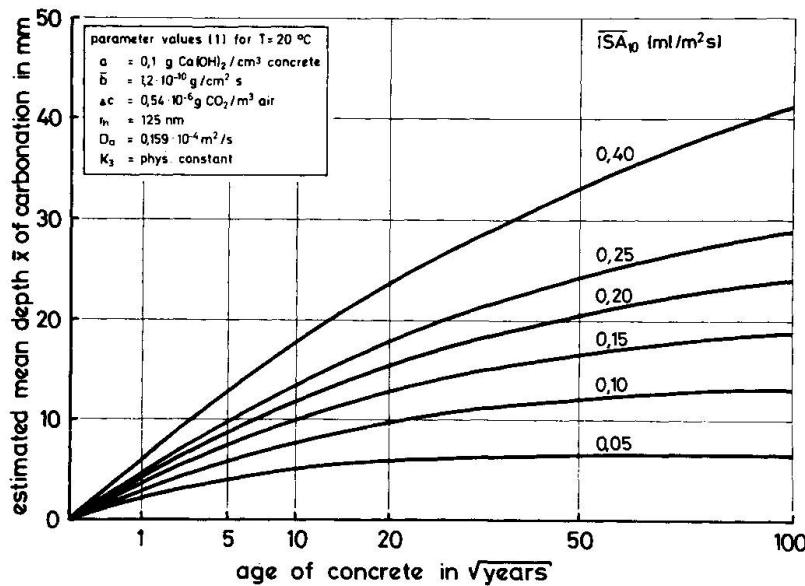
Fig. 1: Mean of carbonation depth dependent on age and  $\overline{\text{ISA}}_{10}$ -value (Equ.(2) and (7))
