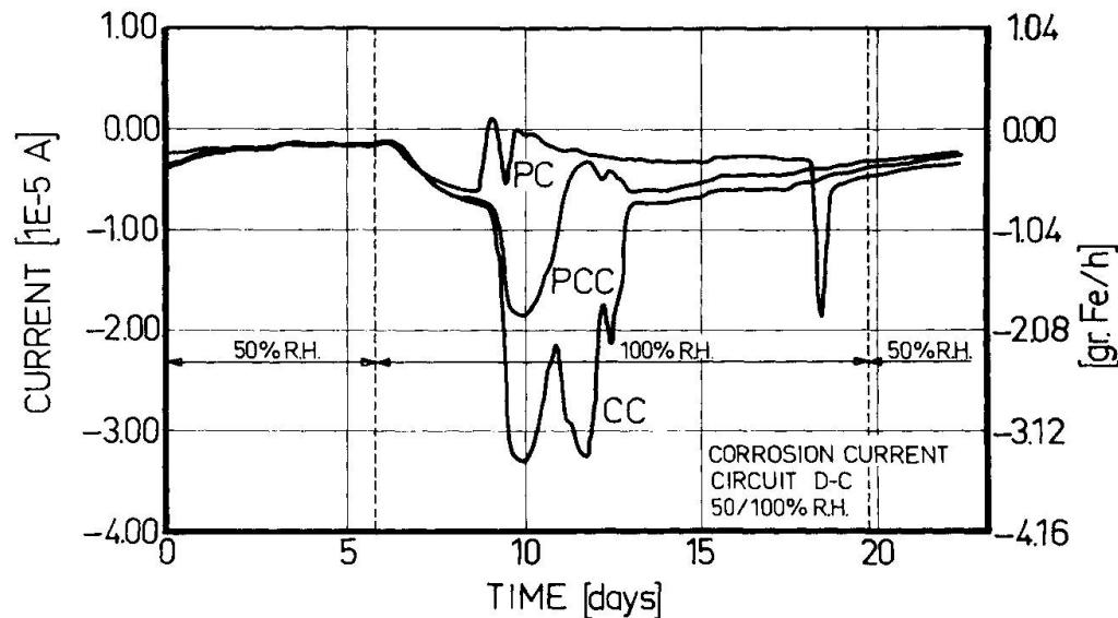
Fig. 5 Corrosion currents for 3 types of repair mortar at 50/100% R.H.
