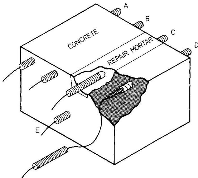
Fig. 2 Concrete corrosion cell
