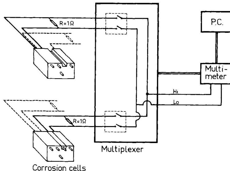
Fig. 3 Measuring system
