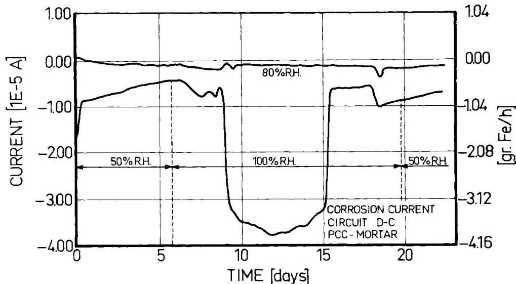
Fig. 4 Corrosion currents for PCC-mortar at 80% R.H. and 50/100% R.H.
