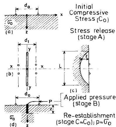
Fig. 2 : Different stages of direct stress measurements, by the release method.
