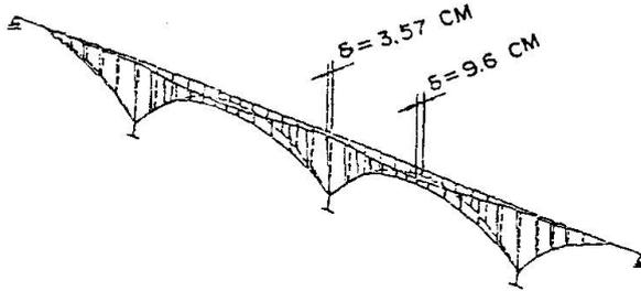
Fig. 4 Horizontal deflection due to horizontal earthquake force.
