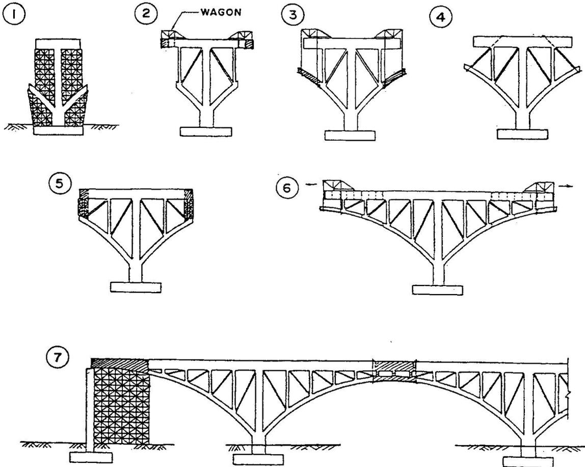
Fig. 6 Erection sequence ( 1. Erection of pier column and first segment. 2. Erection of box girder with moveable wagon. 3. Erection of arch rib with wagon. 4. Placement of oblique constructional PC steel bars. 5. Erection of spandrel strut. 6. Repetition of process from stage 2 to stage 5. 7. Erection of arch crown section with hanging support and end side section with temporary support.).
