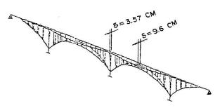
Fig. 4 Horizontal deflection due to horizontal earthquake force.
