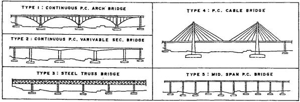
Fig. 1 Five bridge alternatives during the planning stage.
