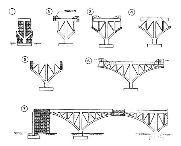
Fig. 6 Erection sequence (1. Erection of pier column and first segment. 2. Erection of box girder with moveable wagon. 3. Erection of arch rib with wagon. 4. Placement of oblique constructional PC steel bars. 5. Erection of spandrel strut. 6. Repetition of process from stage 2 to stage 5. 7. Erection of arch crown section with hanging support and end side section with temporary support.).
