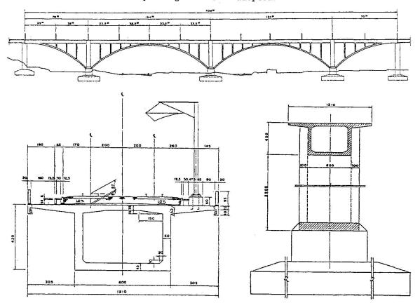
Fig. 2 General configuration of the bridge (Type 1).
